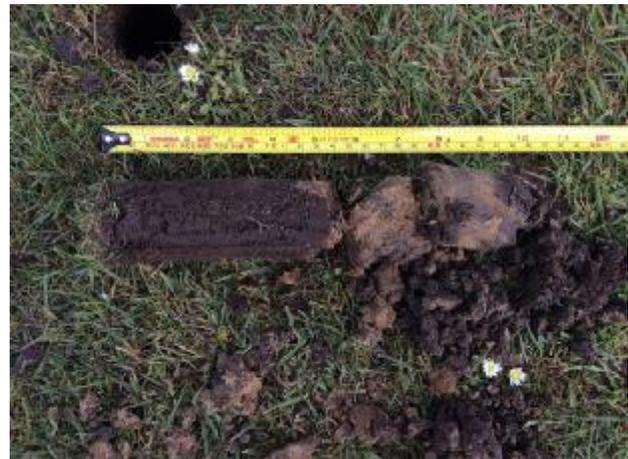
Figure 12: The 8<sup>th</sup> fairway profile is thatchy and organic in the top 125mm.
